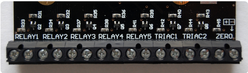
Figure 8: Electrical interface circuitry
