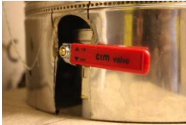
Figure 10.6: Ball Valve Lever Accessibility.
